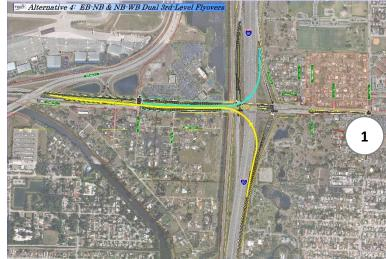
Alternative 4: Dual 3rd Level Flyovers, NB I-95 to WB SR 80 and EB SR 80 to NB I-95: Both the NB to WB and the EB to NB ramps are at the third level. The NB to WB ramp would end east of Australian Avenue but the EB SR 80 ramp to NB I-95 ramp would begin west of the Gem Lake intersection. Keeping both ramps at the third level represents a major cost and time savings during construction, and less visual impacts on the community.
