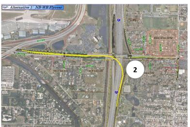
Alternative 1: NB I-95 to WB SR 80 Flyover: Single-lane flyover. The ramp goes over Lang Road and Gem Lake Drive and touches down in the median of SR 80 just east of Australian Avenue. Alternative 1 requires right of way (R/W) acquisition along both sides of SR 80, west of I-95.
