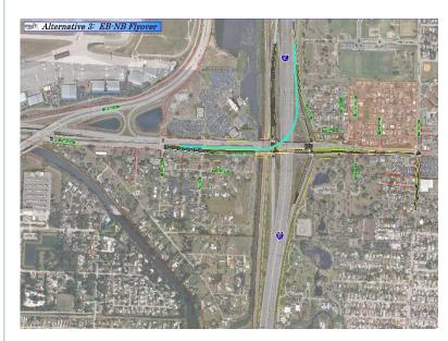
Alternative 3: EB SR 80 to NB I-95 Flyover: Single-lane third level ramp from EB SR 80 to NB I-95. Requires R/W from the south side of SR 80, west of I-95.
